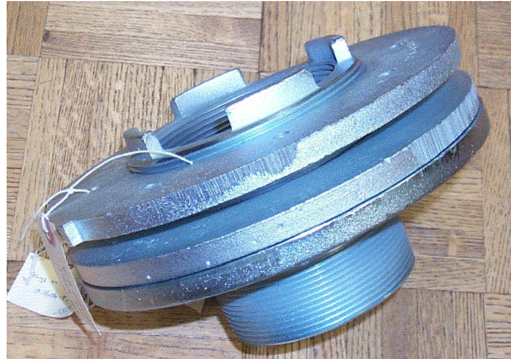
Tank Fitting Adapter (Assembly) - Body, Compression Ring and Washer
